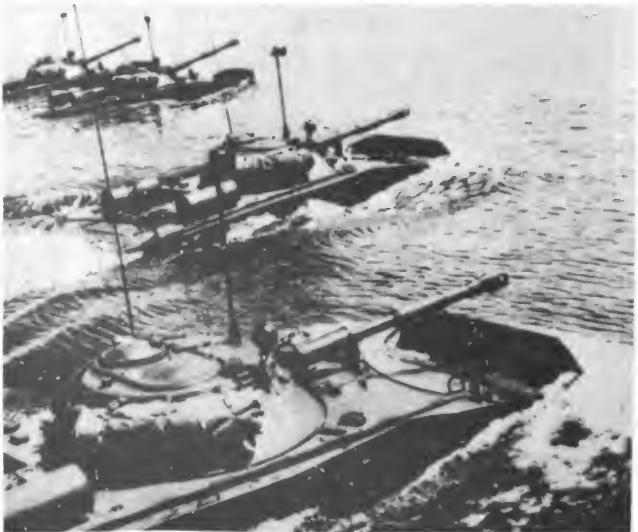
Figure 6-18. PT-76 light amphibious tank. With its light armor and 76-mm gun, the PT-76 is better equipped for reconnaissance missions than for armored battles. Note the rectangular shaped chassis with sloping bow, the low-profile turret, and the fold-up bow flap for amphibious swimming.
